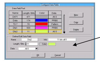
Configure a second data field (11 bits, all bits "0") in the window "Configure Data Fields:
