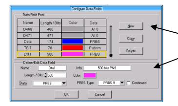
Configure a new data field (500 bits with PN9 data) in the window "Configure Data Fields:
